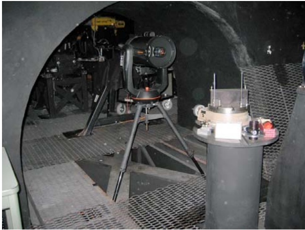
Figures 1 & 2: 280 mm telescope on HJST spectrograph optical bench looking into collimator
